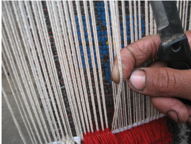
Two warp yarns are held with one finger of the right hand
