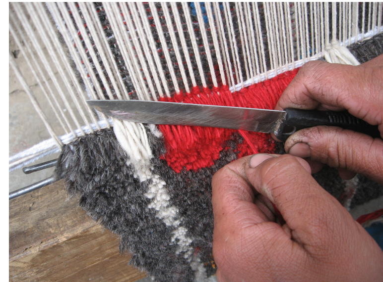
Extra length of pile is cut using a Chaku
