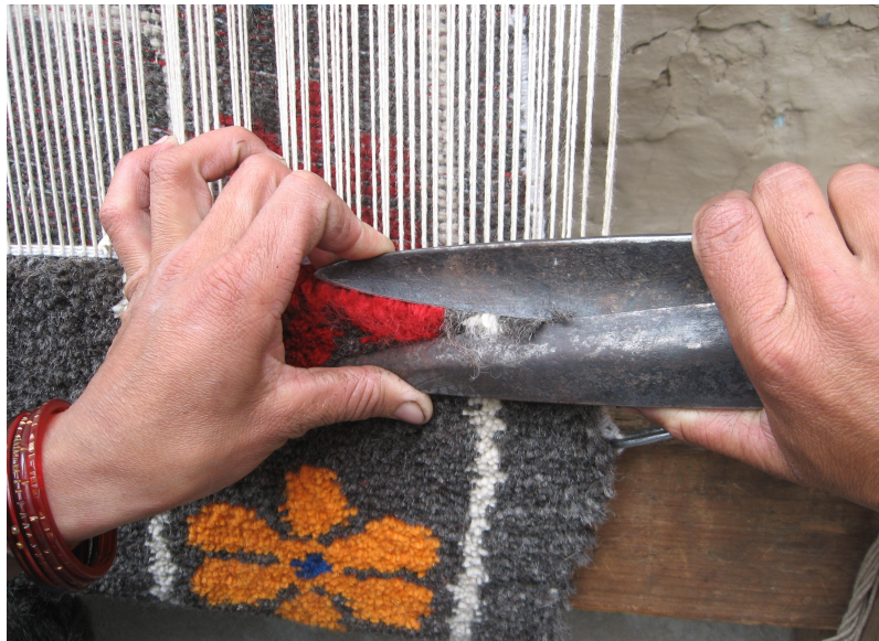
Leveling the pile with Kainchi
