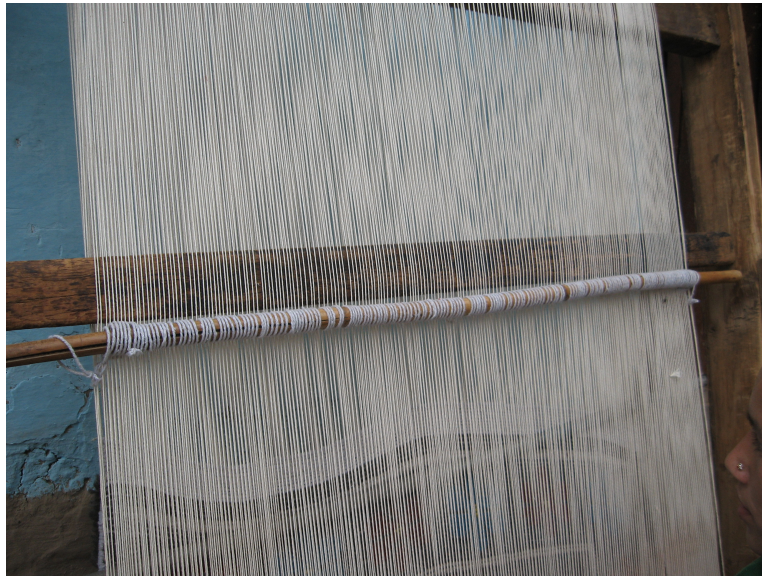
Changing the shed for insertion of weft
