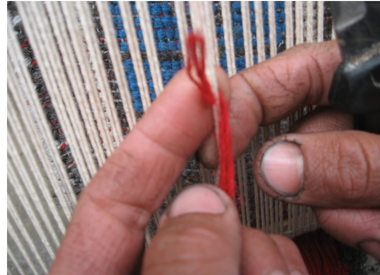
2 ply wool weft is twisted under and then over warp with left finger and thumb
