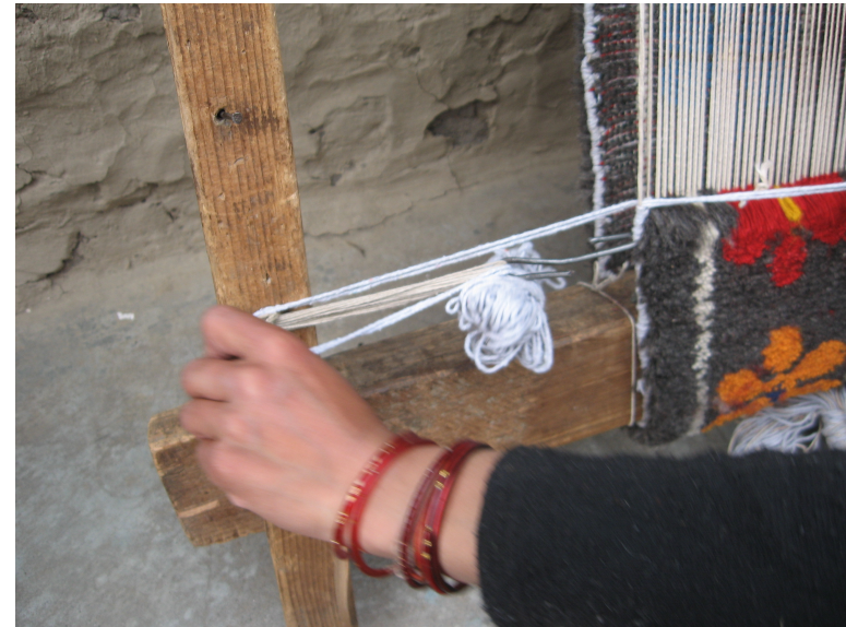
Tying the weft on the hook to bind edge
