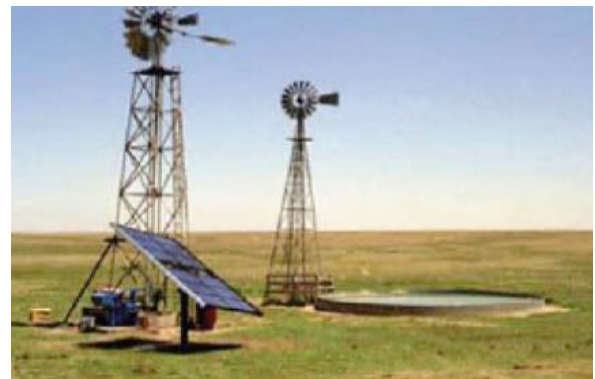
Figure 5 | PV Windmill Integrated Water Pump Source: Chel, A., and Kaushik, G. (2010). Renewable Energy for Sustainable Agriculture. Agronomy for Sustainable Development ; Springer, Vol.31, No.1, 2011, pp.91-118
